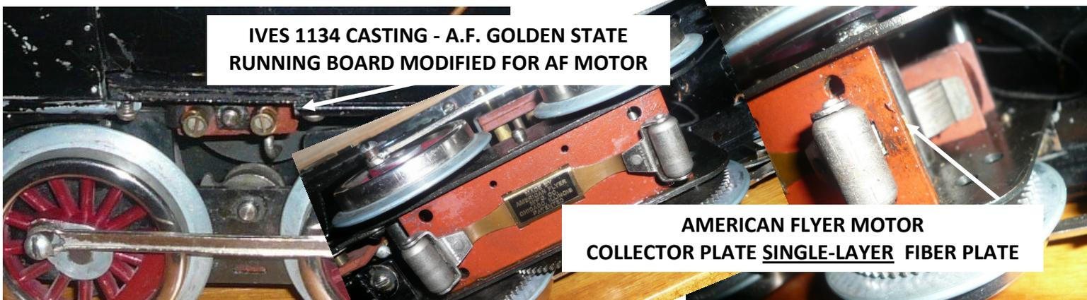
The American Flyer Golden State loco above (modified Ives 1134 casting) is using a pure AMERICAN FLYER MOTOR. In early Flyer production, when the steamers were cast-iron, multi layer fiber collector plates were employed but as soon as the AF used the Ives 1134 casting and 2 years later their own die-cast shell, the single layer fiber plate with metal support tabs was employed.
