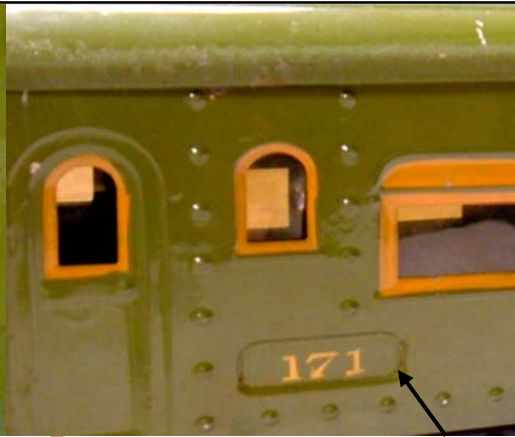
EARLIER 171 WITH OPEN TABS AS COMPARED TO LATER 171 WITH SOLDERED TABS
