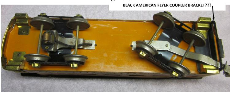
The coupler bracket and steps are riveted only on the front of the 186 cars, and the rear has steps riveted on with no bracket because there is no coupler. The coupler bracket on the lves cars is interesting because it is similar to the coupler bracket used on AF freight and passenger cars.
