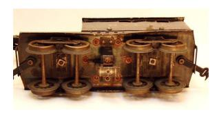
In the middle of the underside of the car is a spring loaded third rail power pickup.
