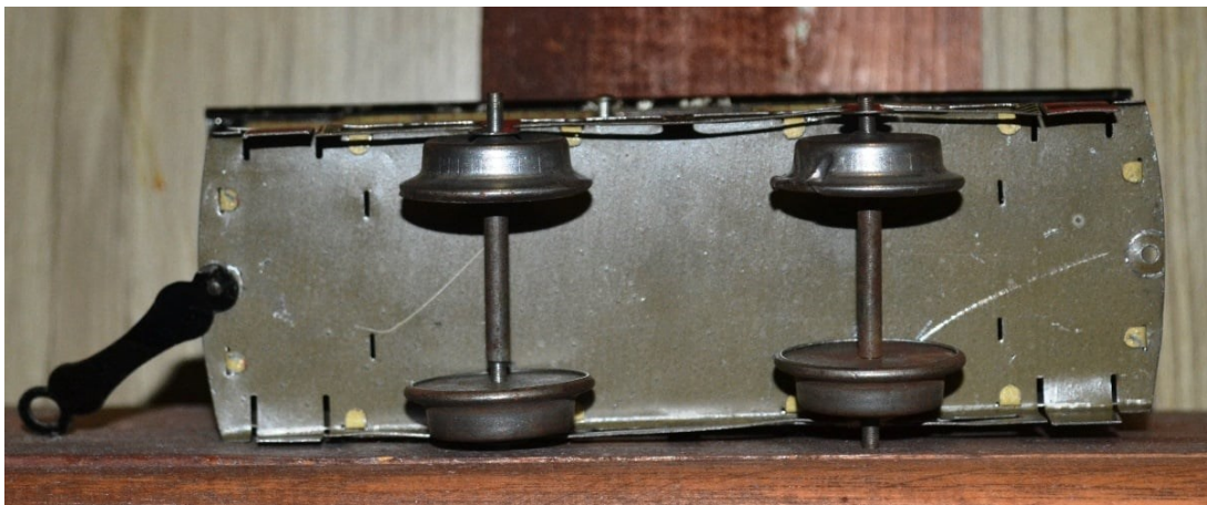
This is a view of the bottom of one of the cars, note they have a single long loop coupler but with tin wheels that have a sleeve over the axle. These are the only two cars I've ever seen with these features and tin wheels, The rest have cast iron wheels
