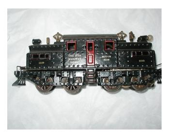
It has a small transformer built into the center cab. The output of the transformer goes to the headlight.
